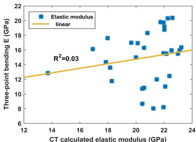
Fig. 4. - Correlation of the elastic modulus calculated from CT mineral density and the elastic modulus found in three-point bending tests is very weak ( $R^2=0.03$ ,  $p < 0.05$ ).
