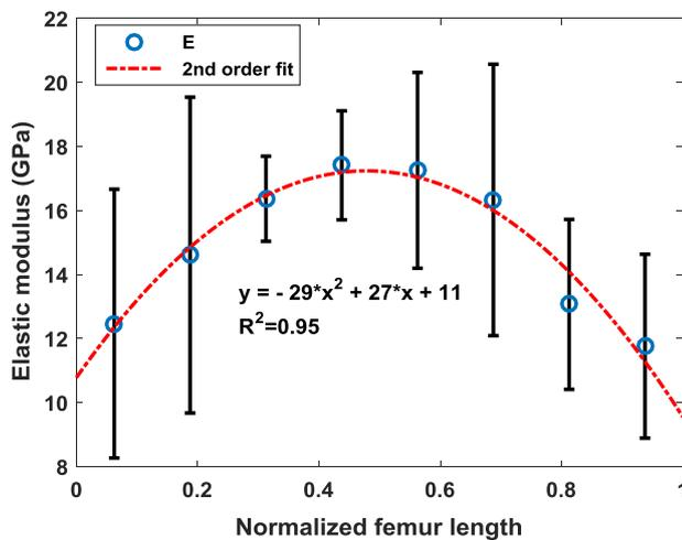
Fig. 5. - Elastic modulus of three-point bending tests is strongly correlated to position along the axis of femur-1 ( $R^2=0.95$ ,  $p < 0.05$ ). Error bars show the standard deviation.
