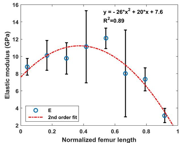
Fig. 6. - Elastic modulus of three-point bending tests is strongly correlated to position along the axis of femur-2 ( $R^2=0.89$ ,  $p < 0.05$ ). Error bars show the standard deviation.
