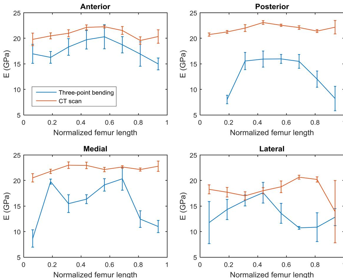
Fig. 3. - Comparing the elastic modulus computed from three-point bending and  $\mu$ CT for different quadrants along the femur-1. As shown, three-point bending results are significantly lower than CT predictions.
