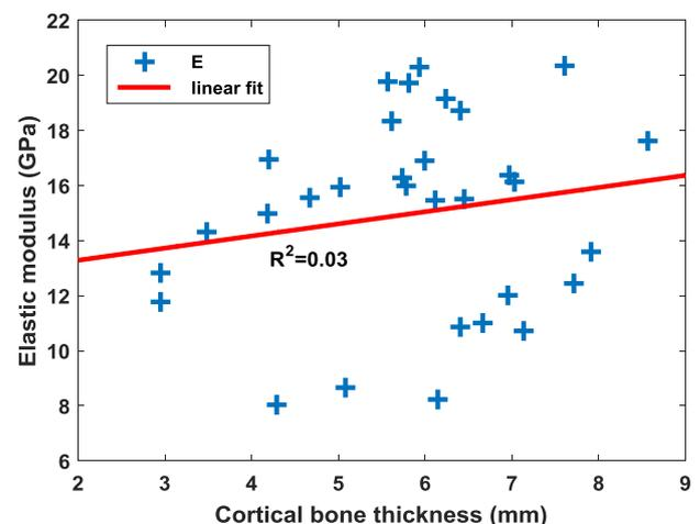
Fig. 7. - Correlation of cortical bone thickness and the elastic modulus for femur-1 is not significant ( $R^2=0.03$ ,  $p=0.35$ ).
