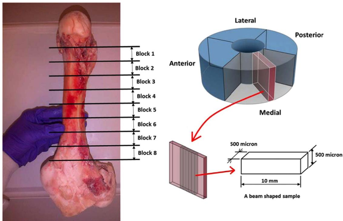
**Fig. 2.** - Left) femur-1 divided into 8 blocks of 2 cm height, Right) One sample block divided into four sections and representation of the bone plate extracted from each block. Five longitudinal beam shaped samples were made out of the bone plate for each quadrant in the block. Block height in femur-2 was 3 cm and each sample's length was approximately 15 mm and 10 mm for femur-1 and femur-2 specimens, respectively.
